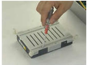
**4. Screw HDD holder on**
