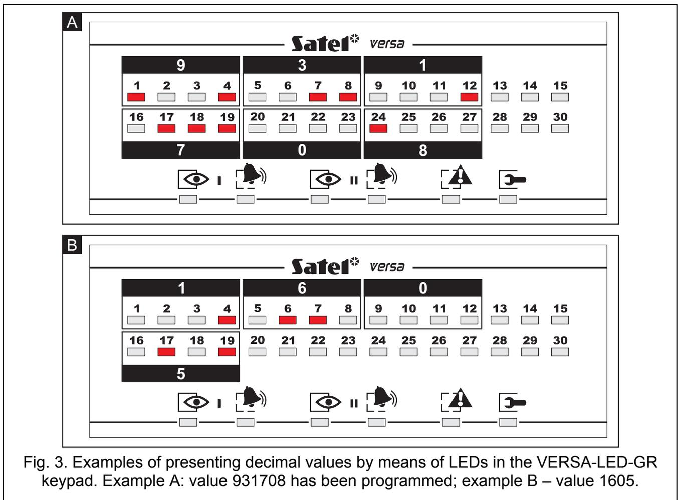
Fig. 3. Examples of presenting decimal values by means of LEDs in the VERSA-LED-GR keypad. Example A: value 931708 has been programmed; example B – value 1605.
