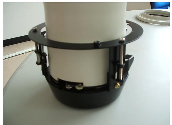
Follow the anti-clockwise direction to take away Speed Dome main body from embedded mount
