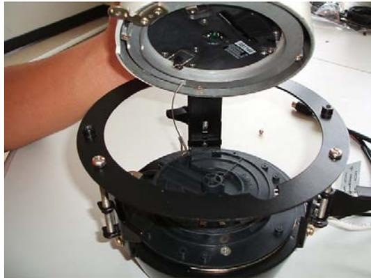
Use screwdriver to drive screws within Speed Dome main body and embedded ring
