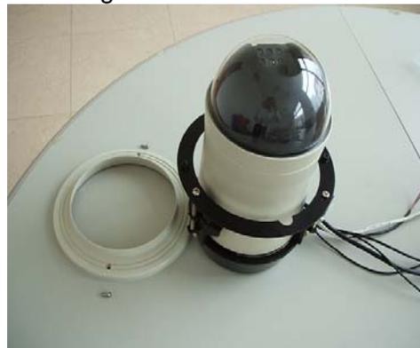
Remove screws from embedded mount and take off this mount
