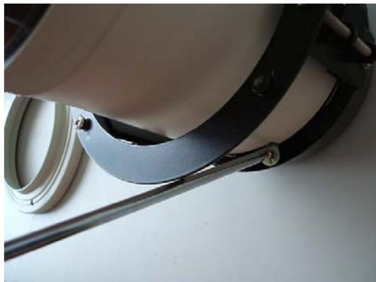
Use magnetic screwdriver to fix the decoration ring with screws. The installation of Speed Dome body is completed.
