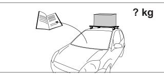
When these roof racks are to be used on a vehicle that is driven off sealed roads, the manufacturer maximum roof load rating (to be found in the vehicles User Manual) should be *halved*. Do not forget to subtract 7.5kg from your maximum carrying capacity due to the weight of the crossbars and legs.
