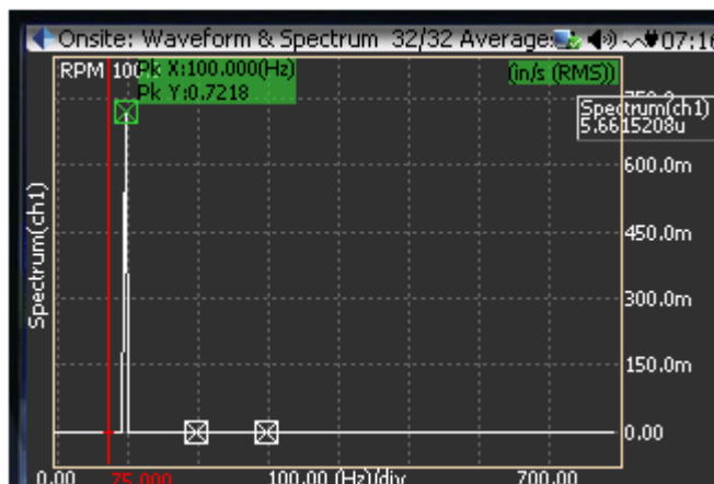
Figure 6: FFT Spectrum in CoCo, in/s RMS
