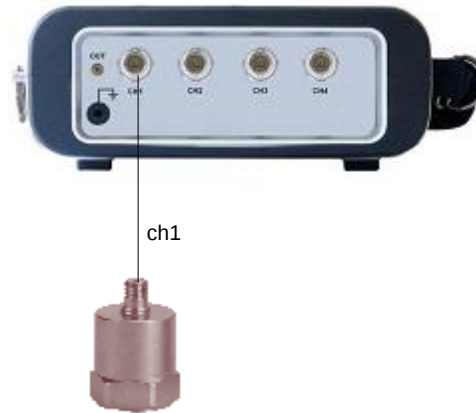
Figure 30: Connecting Channel 1 to Accelerometer
