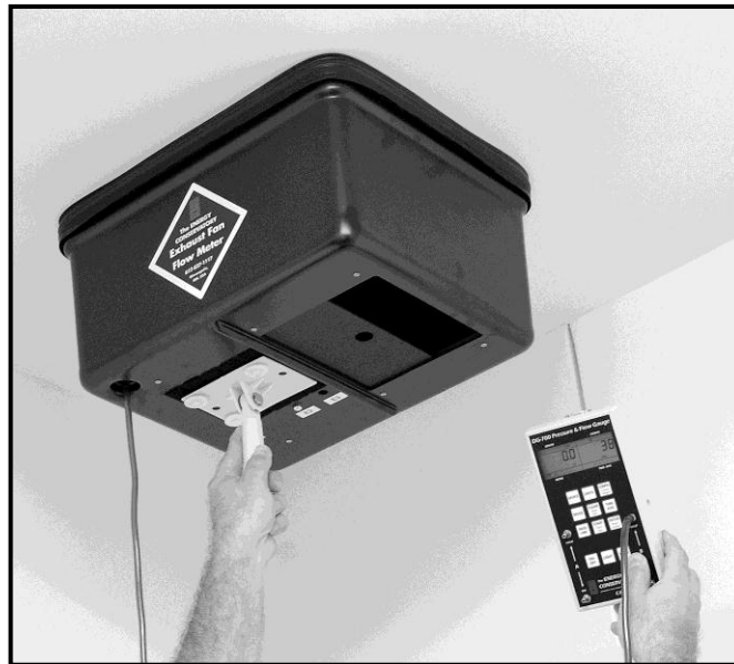
Exhaust Fan Flow Meter with DG-700 Pressure Gauge
