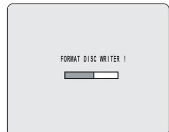
**Operating the DVR (DSR-3716P/3709P)****2 When the still image on the full screen of the playback is displayed, press the [COPY] button.**
