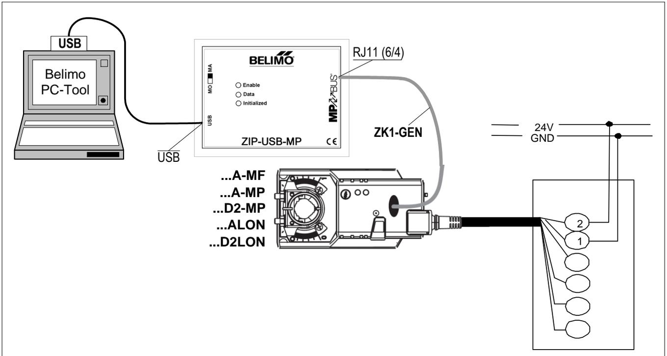
Typical wiring diagram 2
