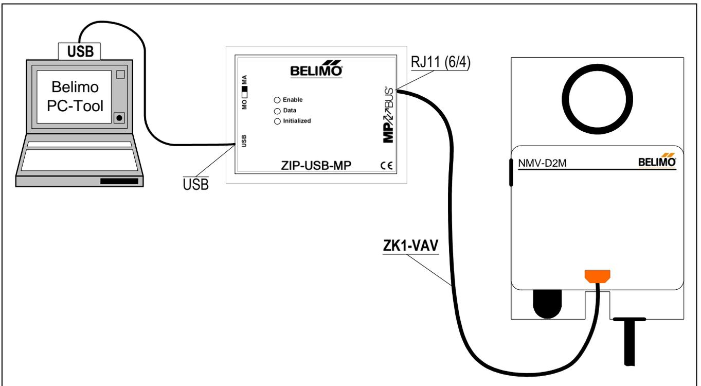
Typical wiring diagram 7
