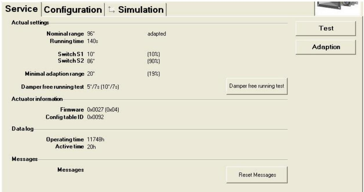
"Service" tab for BF-TopLine fire damper actuators
