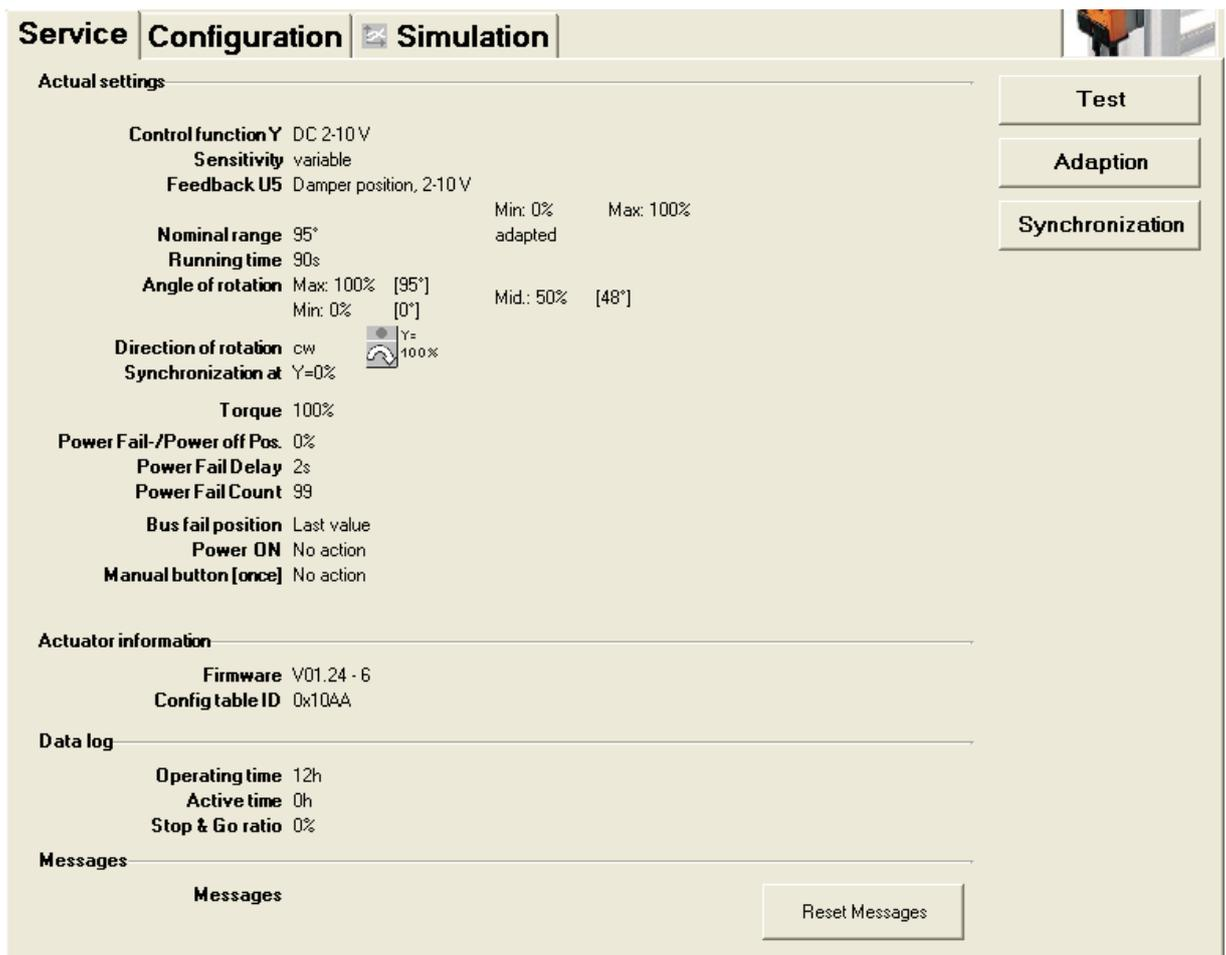
Service tab for full-rotation damper actuators
