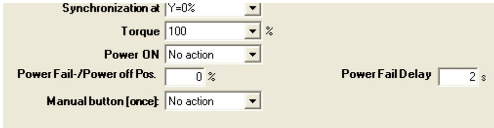
"Configuration" tab for Electronic Fail Safe (excerpt)
