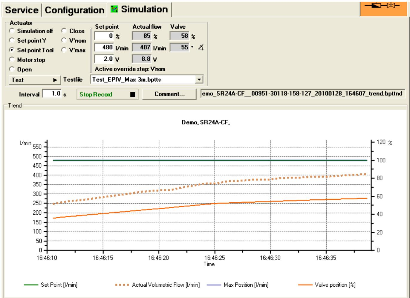
"Simulation" tab for VAV controllers
