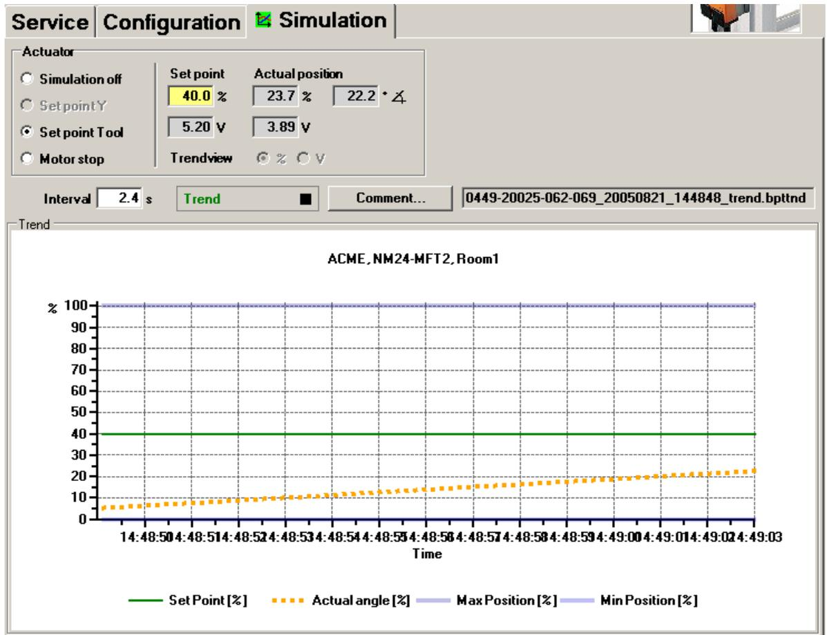
Simulation tab for damper actuators
