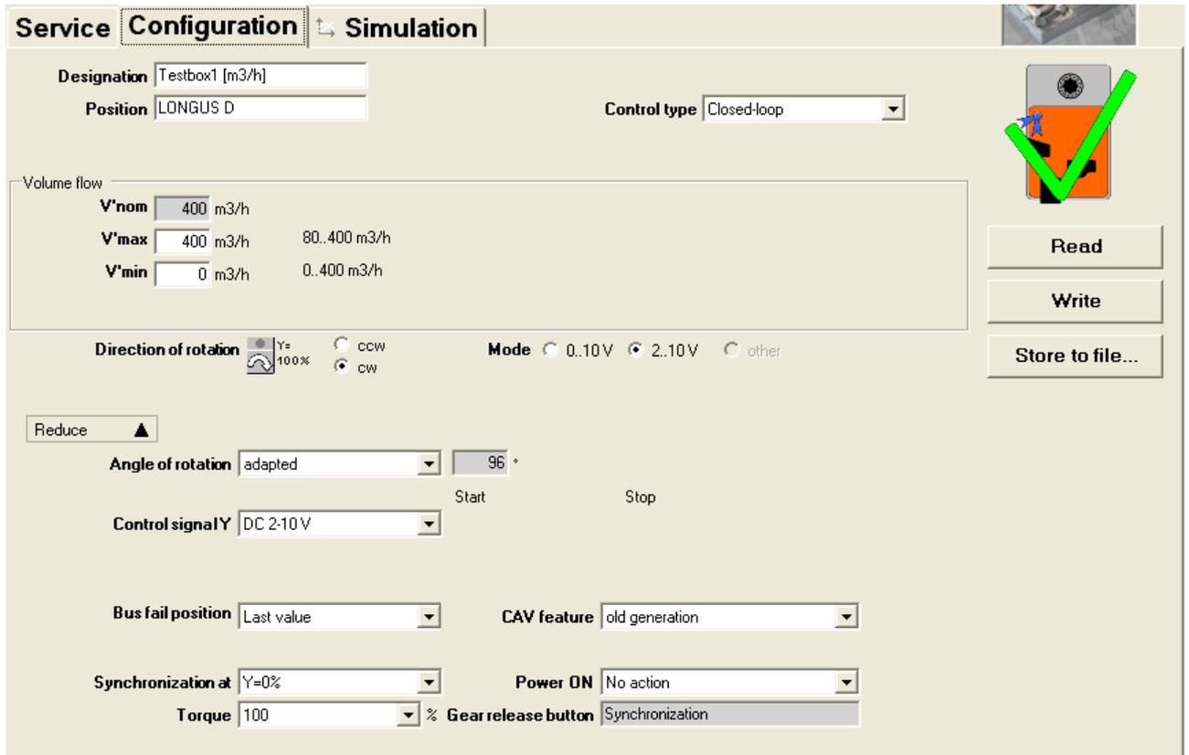
"Configuration" tab for full-rotation VAV controllers
