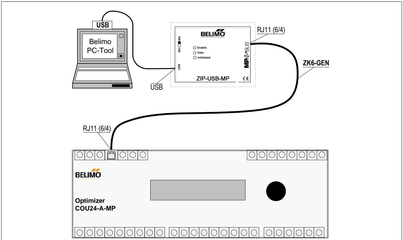
Typical wiring diagram 5
