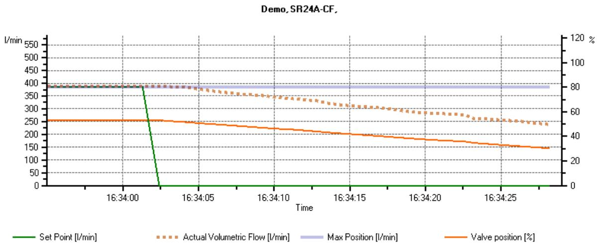
Trend diagram for the control function "Flow control"
