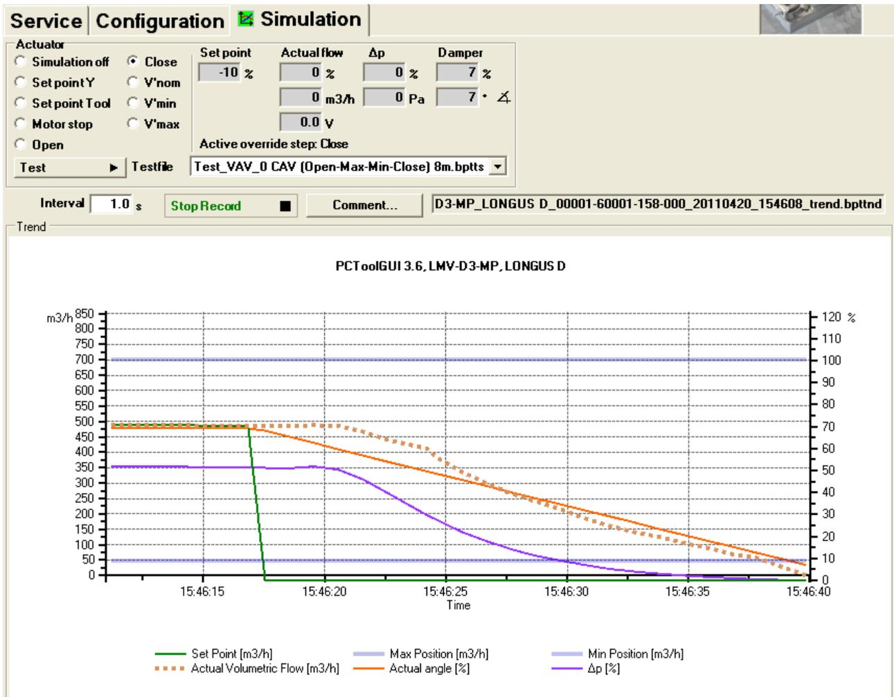
"Simulation" tab for VAV controllers
