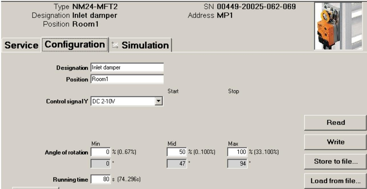
Example of the "Configuration" tab (damper actuator)
