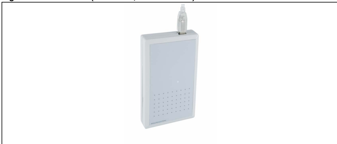
Figure 1. RF reader (ISO 15693, RF 13.56 MHz)
