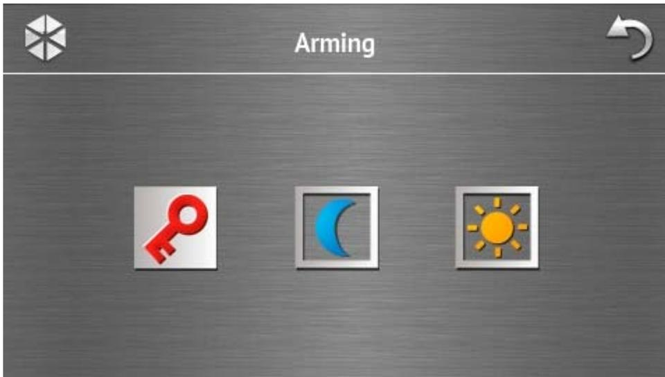
This screen is displayed when you can arm one partition only (also when the quick arming is allowed by the installer in one partition only).
