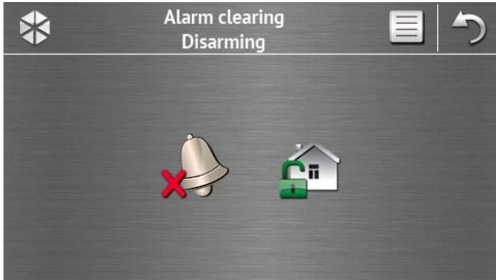
The “Alarm clearing / Disarming” screen will be displayed after you tap the
