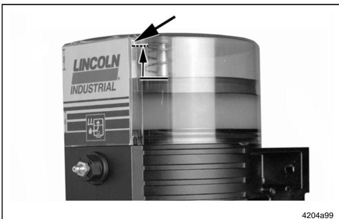
Fig. 10 Vent hole on reservoir
