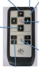
**Speed Settings:** Preset buttons for specific speeds. 1 is the slowest, 4 is the highest. See programing to change speed settings.
