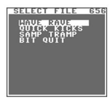
The file operations for the floppy drive make use of the operating system's disk functionality. There are no delete-functions and no replace-and-save options built in. If you try to save the file onto disk using an already existing name the save is interrupted and the drive light flashes.
