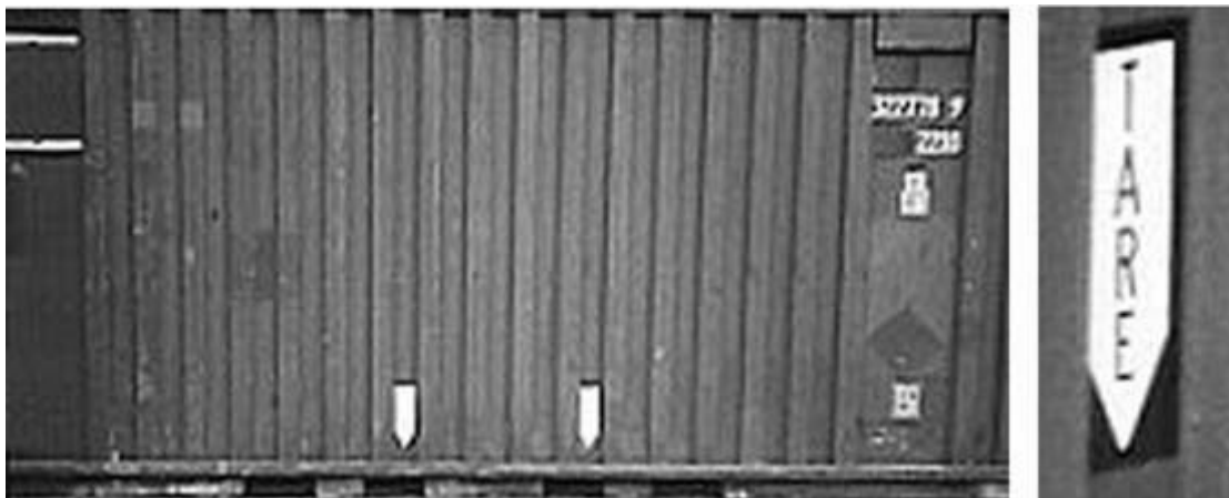
Figure 7-3 The Word “Tare” Used to Indicate Pockets Intended for Empty Lifts
