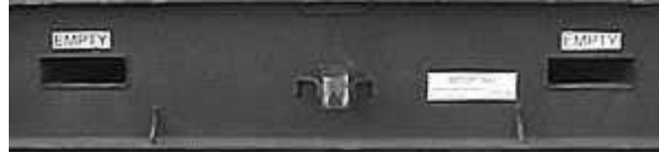
Figure 7-2 Forklift Pockets Clearly Marked for Empty Lifts Only
