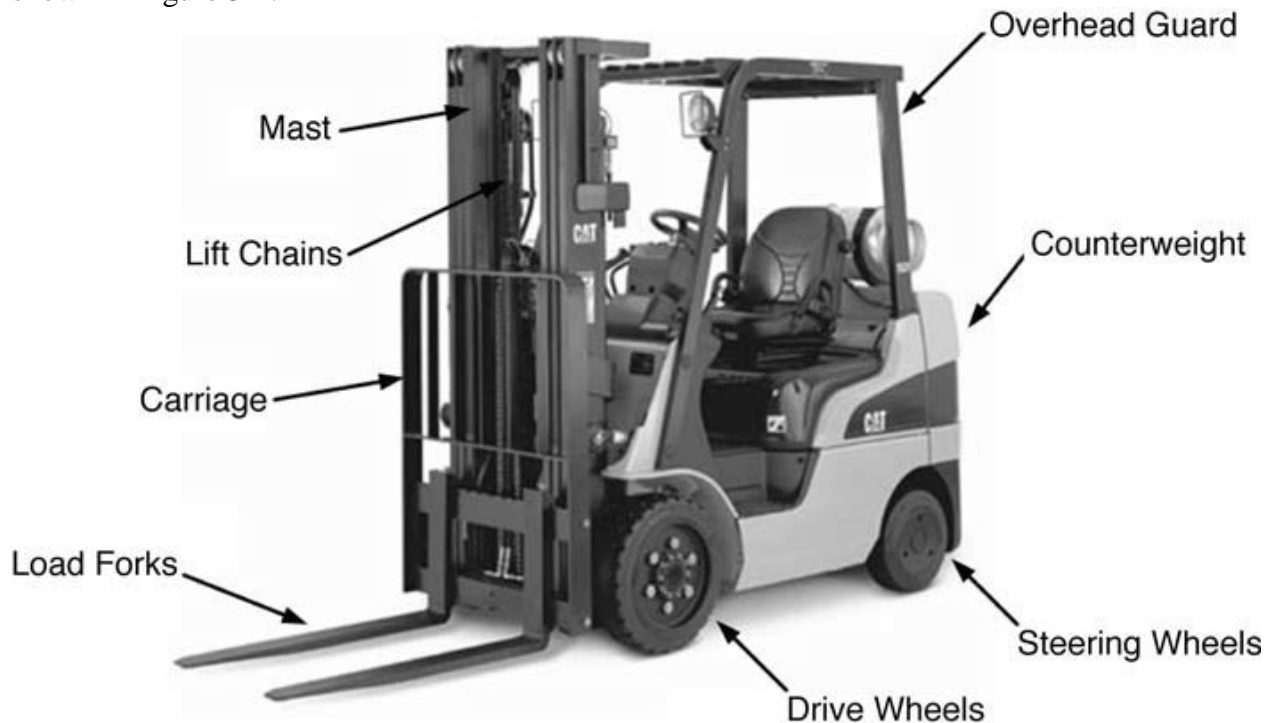
Figure 3-1 Forklift Truck Major Components Photo Courtesy of Cat Lift Trucks
