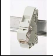
Shielded RJ45-RJ45 feedthrough connector. The keystone latch mechanism maintains the connector in the DIN-rail holder. Adapted for telephony, data and video applications. Occupies 1 standard width on the DIN-rail. Frequently used to bring ports of external devices (phone PABX, data switch,...) to the front panel of the Comm Center cabinet.
