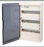
Comm Center cabinet in polymer for wall surface mounting or partially recessed mounting. Fitted with DIN-rails, frontpanel and smoked transparent door. Suitable for small to medium size projects. On the -S22, -S33, -S44 models the frontpanels and side cover of the cabinet can be removed while patch cords stay in place, facilitating add-ons and changes with the system up and running.
