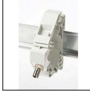
Fiberoptics multimode simplex ST feedthrough connector. The keystone latch mechanism maintains the ST connector coupler in the DIN-rail holder. Occupies 1 standard width on the DIN-rail. The device allows quick termination of Fiber access, backbone or FTTH links in a user premise, industrial site, automation equipment, etc.
