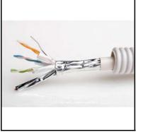
Corrugated 16mm O.D. flex tube pre-equipped with quad-shielded 4 pair cable with one pair optimised for wideband signals. Suitable for high-speed data (up to Gigabit Ethernet), telephony, and wideband audio/video/TV applications. Reduced diameter and bending radius facilitate cable laying and termination in wall boxes. Can also be delivered as bare cable under part. Nr. ABI-KP1003S00.
