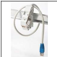
Feedthrough connector with at the front side a universal RJ45 OmniMedia connector with UHF shield. The keystone latch mechanism maintains the connector in the DIN-rail holder. At the rear, a 45cm shielded flylead is terminated by a shielded RJ45 plug. Adapted for telephony, data and wideband audio/video applications. Frequently used to bring the top port of ABI-EL1001S00, ABI-EA1003S00 or ABI-EV1018S00 to the front panel of the Comm Center cabinet.
