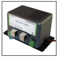
The HiFi amplifier boosts the music signal coming from the DMS Radio & Control Module and can be fitted in the close proximity of the in-wall or in-ceiling speaker. Alternatively it can be housed in a central comms cabinet. The unit is a single building block with built-in mains power supply. The amplifier's power supply also feeds the Radio & Control Module with 12V DC power. A pair of 22 Watt amplifiers are adequate to provide a large room and high quality speakers with true HiFi stereo sound.
