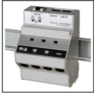
The ABI-ET2003S00 is a passive splitter module for the distribution of analogue (PSTN) phone and ADSL signals. An external ADSL filter is no longer needed thanks to the built-in filter. This simplifies the installation and comissioning of phone, fax and ADSL modem-router. The ABI-ET2003S00 does not provide the call-confidentiality function.
