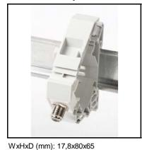
Ensures a quick termination of connectorised coaxial cables in the Comm Center cabinet. The keystone latch mechanism maintains the connector in the DIN-rail holder. Adapted for wideband audio/video applications. Frequently used to bring coaxial ports of modules ABI-EV10xxS00 to the front panel of the Comm Center cabinet.
