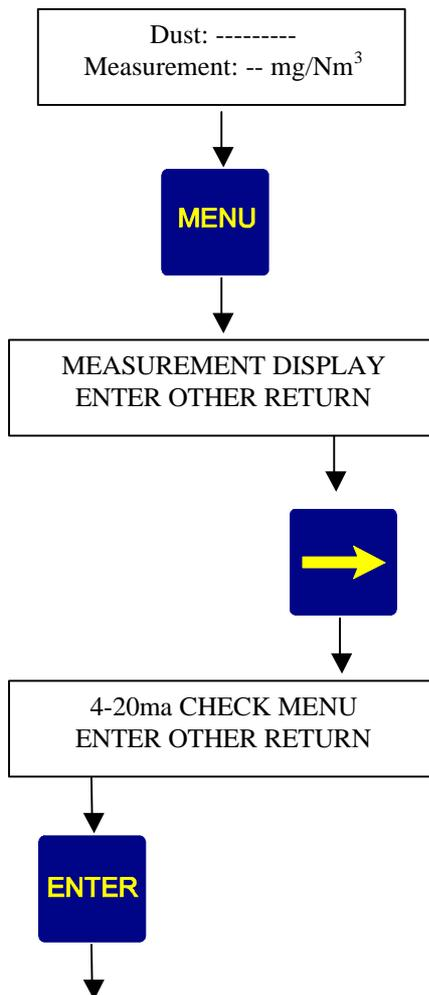
Press this key 6 times until the "Checking the 4-20mA" menu appears
