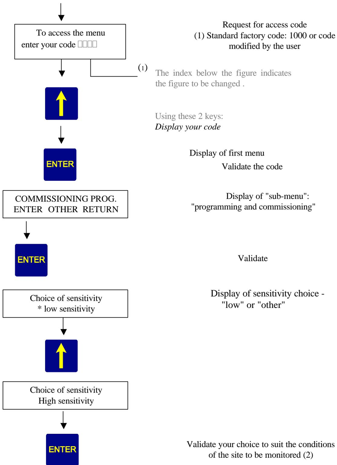
(2) **Note:** the sensitivity is chosen as a function of two parameters: the level of sunshine and the level of alternating signal.
