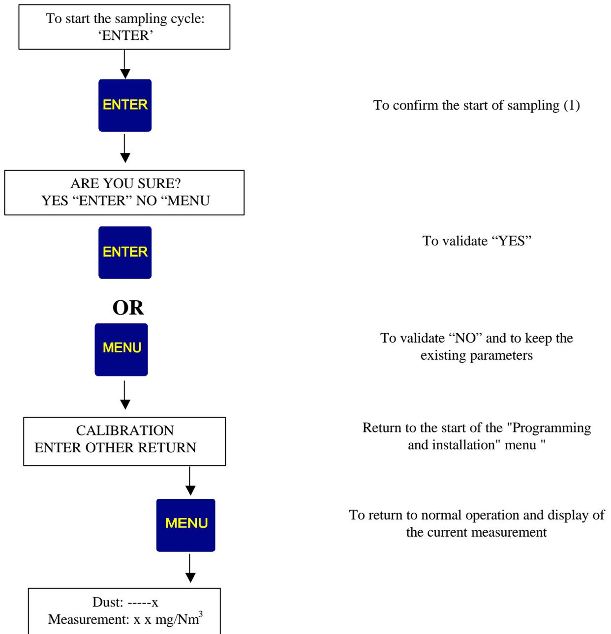
(1) When the "start of sampling" is confirmed, the EP1000A stores the measurements (storage in memory) until the moment when "end of sampling" is validated.
