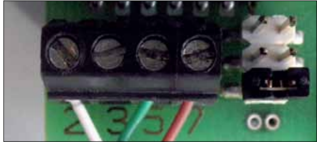
Fig.9 Connection on SMA-RS485 piggyback
