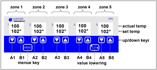
The set temperature can be adjusted by pressing the up- and down-keys at each zone. You can switch between the three operation modes by pressing the two keys (A and B) of a zone simultaneously.(See chapter 2.4)
