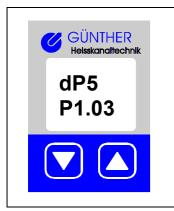
After switching on, the controller's left LED display (zone 1) shows the start report: the top line indicates the number of zones connected to the controller (DP5 - five zone controller); the bottom line indicates the number of software version. After the start report, the DP3/DP5 automatically runs a system check then starts the operating mode.
