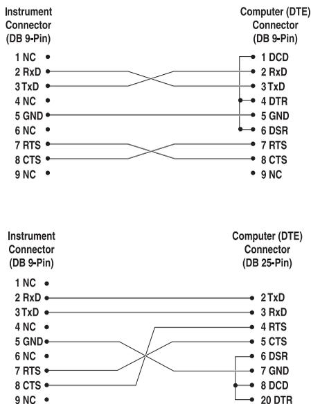
Figure 10 Serial Cable Wiring
