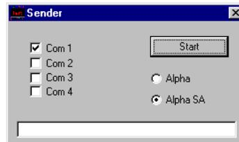
3. The application will send out test messages to every sign on the network, that is, signs with addresses 1 through 255. It starts with message 0 (zero) and goes to message 999 and then repeats the cycle as long as it is running or until the *Stop* button is clicked.
