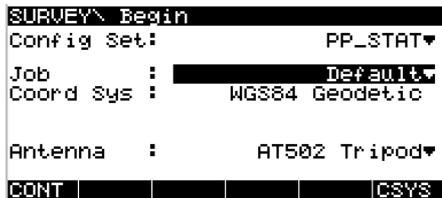
Some basic decisions have to be made in this panel: Which configuration set should be activated, which job the raw data should be stored and which antenna set-up should be used.
