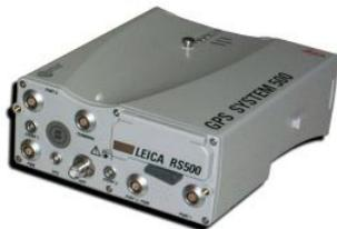
The RS500 uses the same housing and meets the same technical and environmental specifications as the SR5xx sensors. For details please refer to the Technical Specifications section of this manual.
