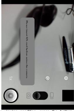
Under viewing condition, press the bottom icons to do the following operations. Press the left icon to capture a picture or film a video, scroll the middle icon to switch between camera mode and video mode. The right icon shows the currently captured picture or video.
