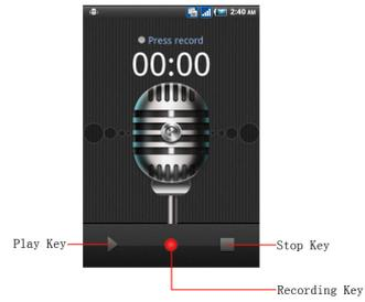
Press Recording Key to start recording. In the middle of the screen is a timer. Press Stop Key to stop recording and select "Save" in the popped out "Save/Cancel" option to save the record. You can press play key to listen to the record before selecting "Save/Cancel".
