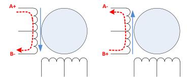
A stepper motor with four wires is not much different from one with six wires. The middle taps of the coils are missing:
