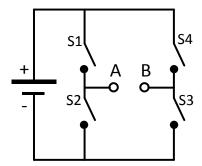
The two contacts in the middle A and B can be connected up to a DC motor.
