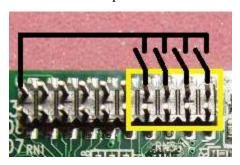
You can connect a switch which is normally open and gets closed if the end-stop position is reached. In that case you must program the end-stop as active low.
