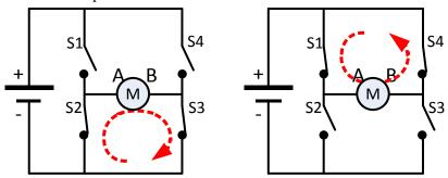
These are what is called 'braking' scenarios. The motor is shorted which mean any residual current in there can flow and will cause the motor to brake. The Gertbot does not support these two modes.
