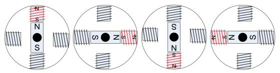
In reality the internal of the motor is much more refined, with many small teeth and two sets of teeth on the rotor. The two sets of teeth are slightly offset and the magnetics are controlled in such a way that the rotor switches from one set of teeth to the other.
