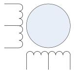
To generate a magnetic field you have to send a current through one if the coils. There are several ways of doing this. Here we connect the middle of a coil to the + and then we can use two switches to enable either one or the other coil.
