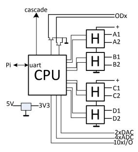
The four H-bridges can be used to control either four brushed motors or two stepper motors or two brushed and one stepper motor. You talk to the board using the UART (serial port) which must be set to 57600 baud, 8 bits 1 start, 1 stop bit, no parity.
