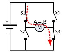
We see that the current is flowing through the motor from A to B. This will cause the motor to rotate.
