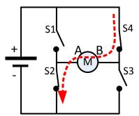
We see that the current is again flowing through the motor, but from B to A just the opposite direction than in the previous picture. Thus the motor will also rotate in the opposite direction.
