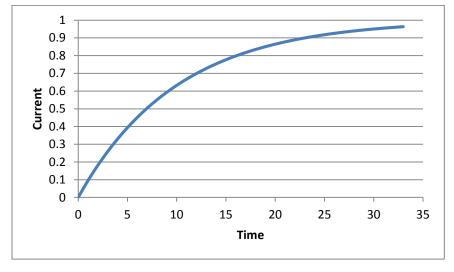
At time t=0 we close the switch. The current starts to rise and after a while it gets to its maxim value. The time that takes depends on the motor coil. In a small coil it can happen in a few microseconds, a large coil can take several milliseconds to reach the maximum current.
