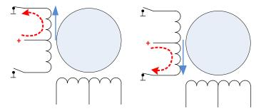
The blue arrow indicate the direction of the magnetic field. As you can see the two operating modes have opposite magnetic fields. I have not drawn it, but you can imagine that the same is possible with the coil at the bottom. The advantage of this method is that you need only two switches to flip the magnetic field of the coil around. But the disadvantage is that you use only half of each coil. For two sets of coils you need four switches.
