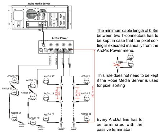
If the line between ArcDots is disconected, the ArcDots behind point of interrupt will not work. Before restoring connection between ArcDots, switch off the ArcPix Power.
