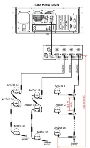
Every ArcDot line has to be terminated with the passive terminator!
