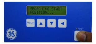
4 Release the **GO** button when the LCD display shows **READY TO CAL?**.
