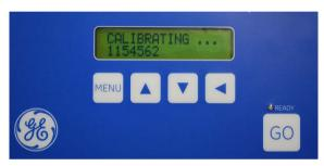
The jaws will close to approximately 5 mm apart and then start moving together slowly. The LCD display shows the incremented position count information.
