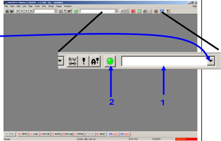
**6 - *Note:* If, when starting Vision, the communication button **(2)** is yellow, communication must be disabled by clicking on it (the button turns red), before selecting the ECU.**
