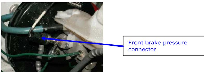
**Note:** The front brake pressure connector is positioned under the windshield aperture on the standard wiring.
