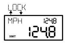
the currently displayed speed to the main window. If Peak mode is on, all speeds just freeze in their respective windows. LOCK alternately displays in the upper left message window. Press the trigger a second time to unlock the readout. This function is useful if the operator needs to manually hold readings.
