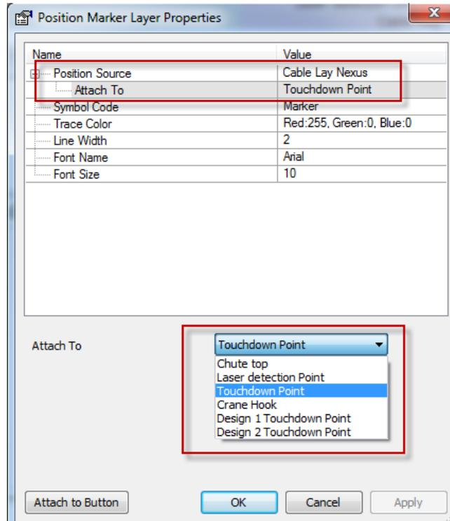
Figure 3-23 Position marker layer properties
