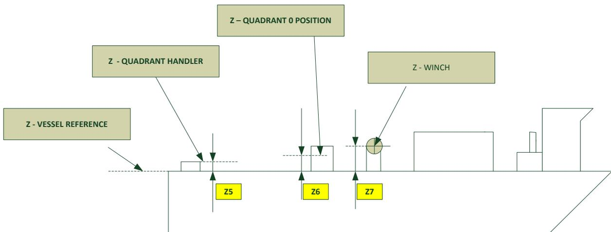
Figure 2-10 Vessel reference Z (side view)
