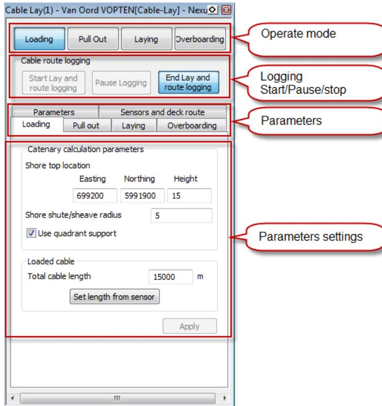
Figure 3-2 Functions cable Lay Control
