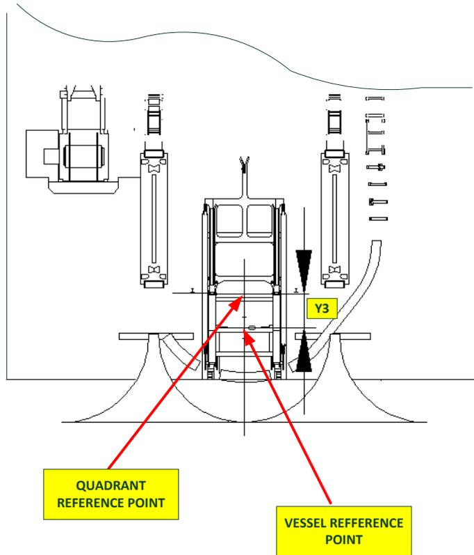
Figure 2-9 Quadrant handler reference point (top view)
