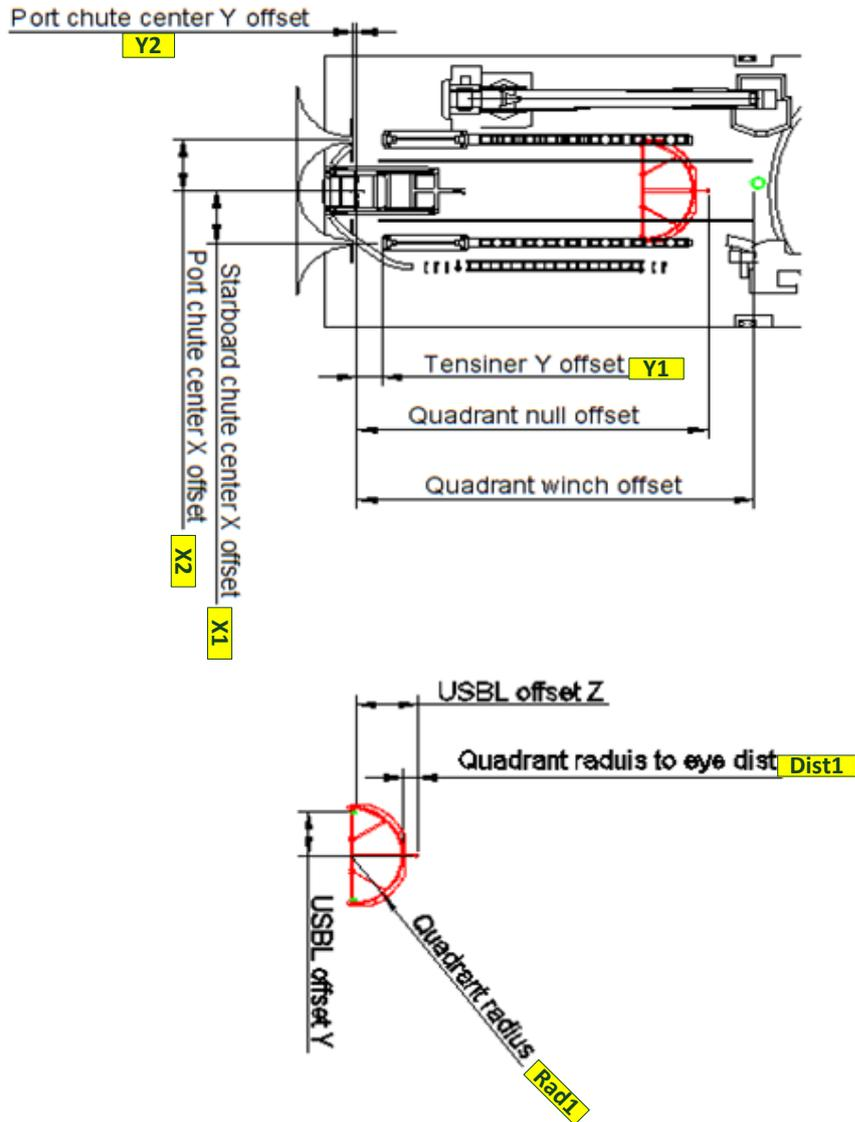
Figure 2-1 Offset/Dimensions chute, tensioner and quadrant
