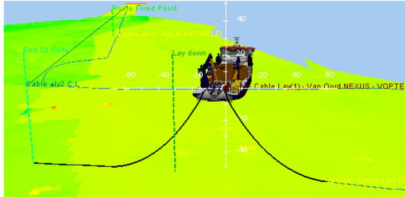
Figure 4-12 Teklink and cable: two catenaries
