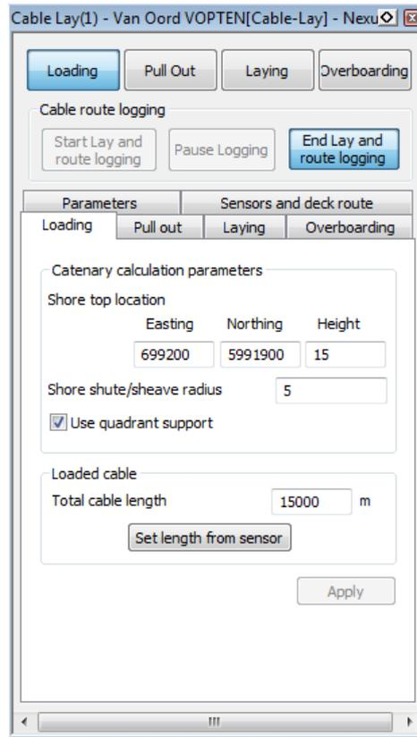
Figure 3-1 Cable Lay Control View
