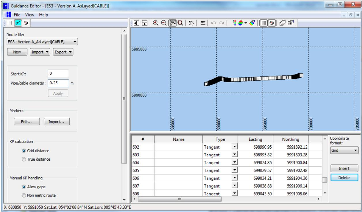
Figure 4-15 Guidance editor with cable as layed route.
