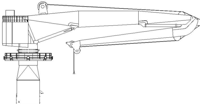
Figure 2-4 knuckle-boom crane
