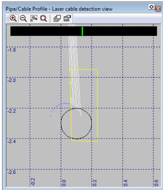
Figure 3-32 Example of a laser cable detection view with a defined polygon.
