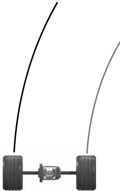
Figure 2-23. During Turns the Wheels Cover Different Distances
