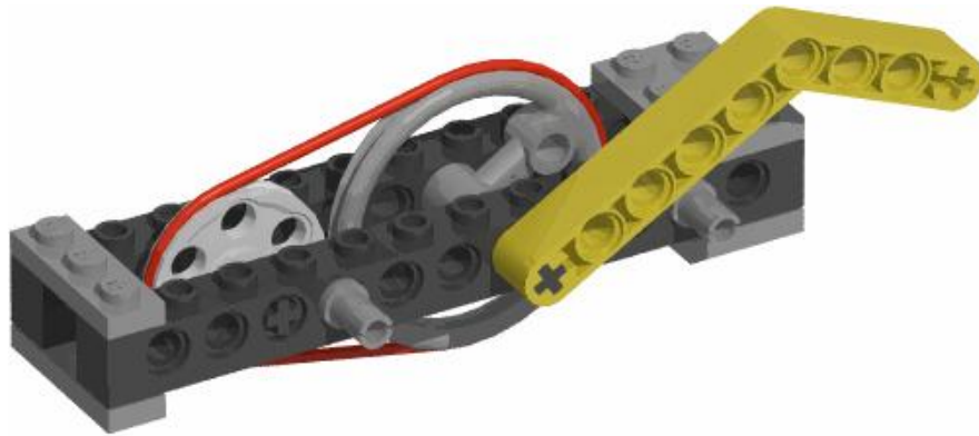
Figure 2-31. Using Pulleys to Limit Torque
