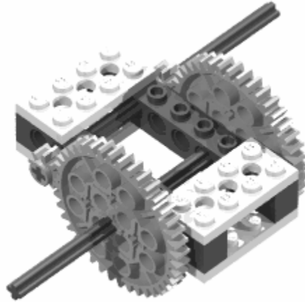
Figure 2-36. Split gear made from LEGO
