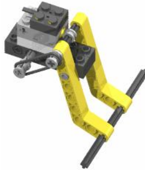
Figure 4-13. A Normally Closed Bumper Design
