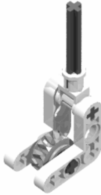
Figure 2-17. A Small Wheel Built from Two 12t Bevel Gears
