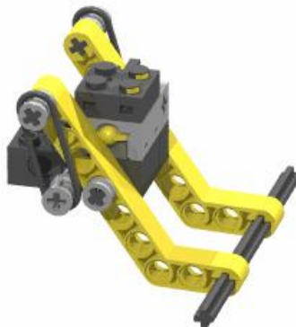
Figure 4-14. Improved Normally Open Bumper
