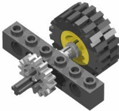
Figure 1-8. A Typical Driven Wheel Assembly
