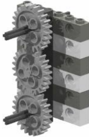
Figure 2-5. Circumventing Vertical Gear Spacing Restrictions
