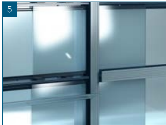
5.1. Once the vertical pressure plates are fixed, the horizontal pressure plates can be fixed into place, remember to allow 2 mm gap between horizontal pressure plates & vertical pressure plates as the vertical covers will not clip on properly.
