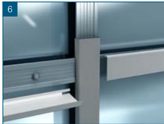
6.1. The vertical covers can now be clipped in over the pressure plates, followed by the transome covers. Remember to position the horizontal covers correctly with the weep holes on the underside. Always ensure that the vertical covers are fitted past the transomes.
