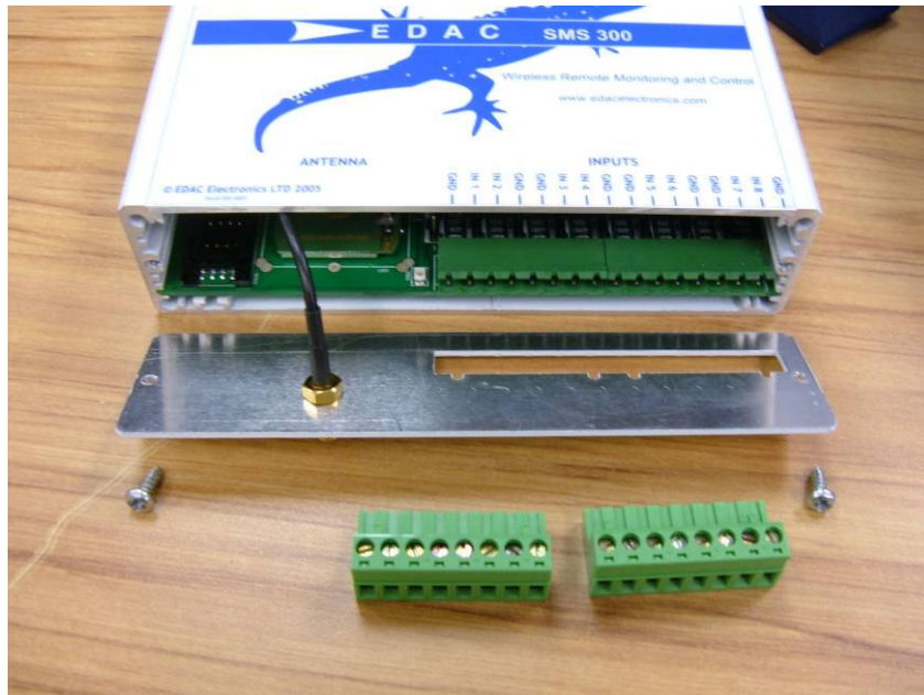
Fig 3.1.2a Removing terminal blocks and end plate
