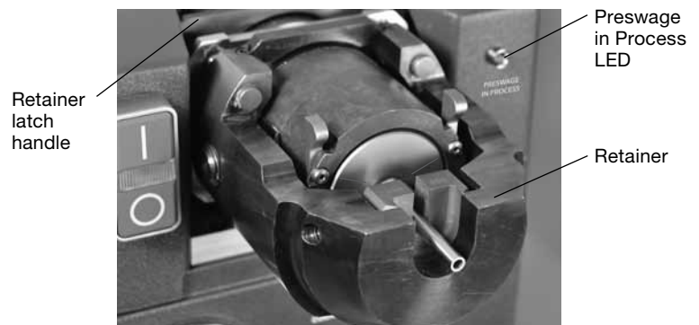
Fig. 14 Preswaging the Tubing
