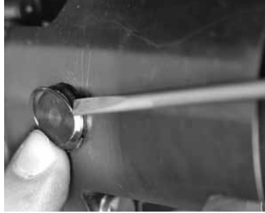
Fig. 20 Removing Clips from Retainer Shaft
