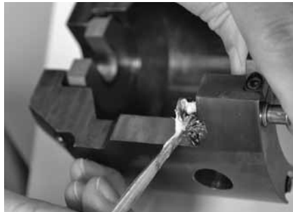
Fig. 23 Applying Lubricant to Latch Pins
