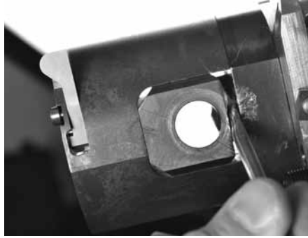
Fig. 22 Applying Lubricant to Connector Shaft
