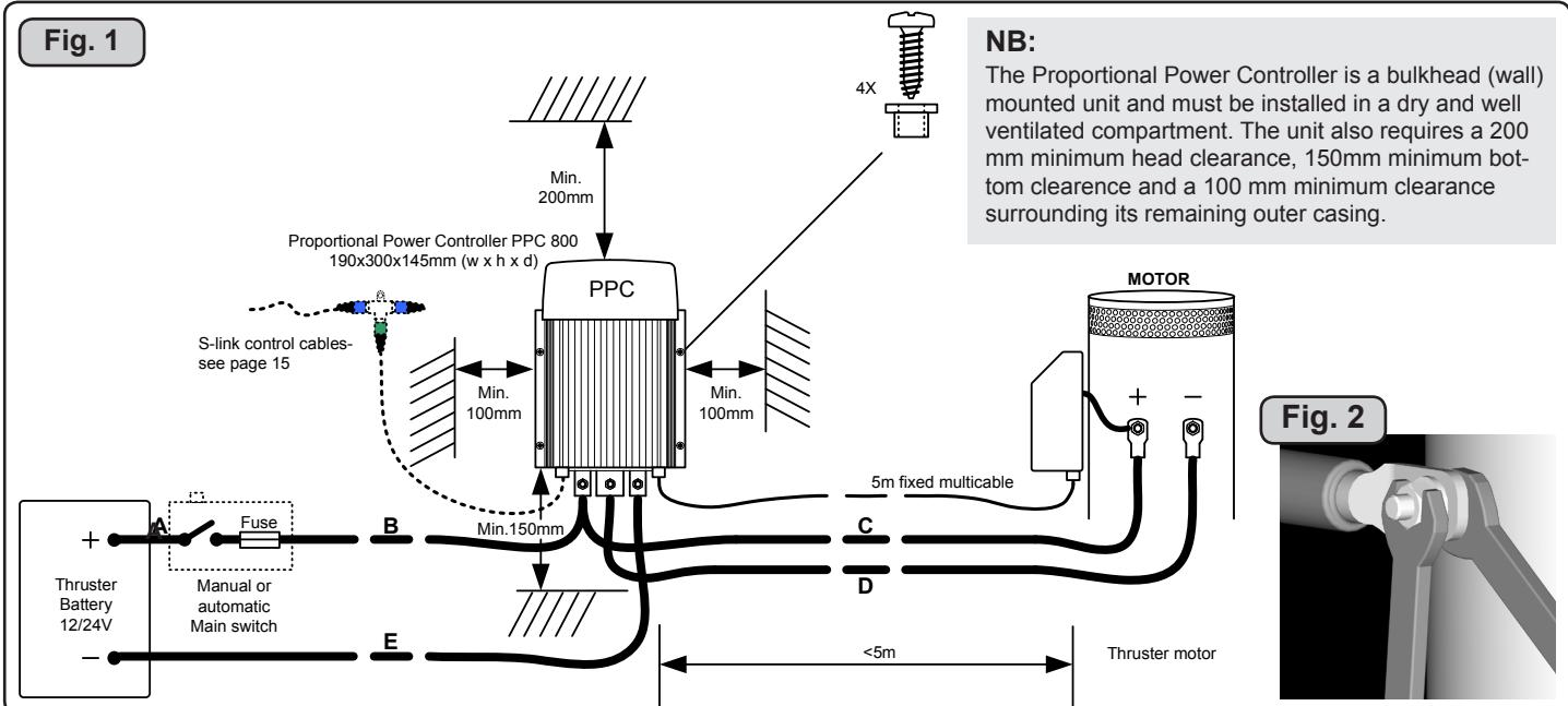
Refer to the manual for the specific thruster used for correct sizing of battery capacity and cable dimensions.
