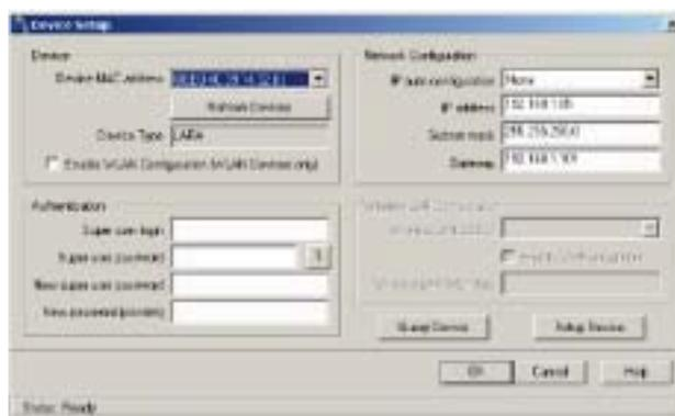
On the upper left corner, the MAC address of the IP-KVM switch is displayed. To detect the MAC address, manually, press the button “Refresh Devices”. The displayed MAC address is the same MAC address printed on the white sticker placed on the back of the IP-KVM switch. If the IP-KVM switch is connected via USB, it is classified as an USB device and an appropriate drive letter is chosen for this device.
