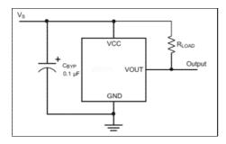
If you are not using a Zaber controller, ensure that your controller has a pull-up resistor on the output line of the Hall sensor as shown in the diagram. The bypass capacitor is optional, but may help to eliminate false triggering in noisy environments. The typical value for the pull-up resistor ( $R_{LOAD}$ ) is 10k and for the bypass capacitor is 0.1uF to 1uF. The larger the capacitance, the better the noise filtering but the slower the response time.
