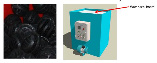
Fig.C3: The plastic Bio-Filtration ball and water seal board.
