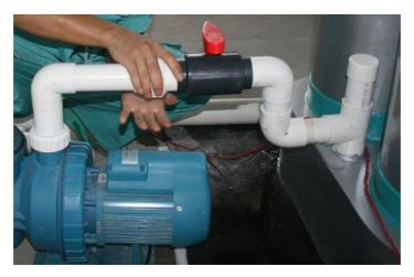
Fig.C8-3 Pipe between the Pump and Flowing-sand bioreactor.
