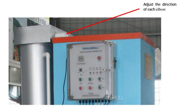
Fig.C5: Adjust direction of water inlet (elbows)
