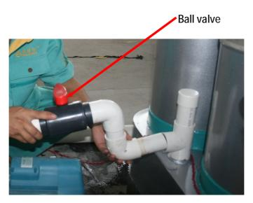
Fig.C8-1: Pipe between the Pump and Flowing-sand bioreactor.
