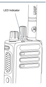
**Blinking green** – Radio is receiving a non-privacy-enabled call or data, or detecting activity or retrieving Over-the-Air Programming transmissions over the air.
