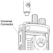
Insert the hooked end of the cover into the slots above the universal connector. Press downward on the cover to seat the lower tab properly into the RF connector.
