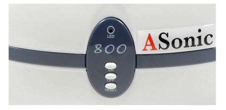
On the top of control panel is red LED indicator light for utlrasound operation. In the middle are "ON" and "OFF" buttons fora activation and deactivation of ultrasound. On the bottom is the button "RESET" which will reset the timer to starting value of 180 seconds.
