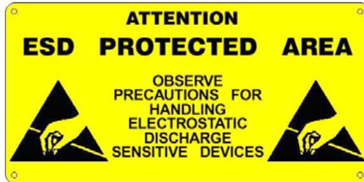
Pins of Modules are not provided with any kind of ESD protection. They are connected directly to their respective pins of microcontroller. Modules are affected by electrostatic discharges. Personnel who handles Modules is invited to take all necessary precautions to avoid possible damages caused by electrostatic discharges.
