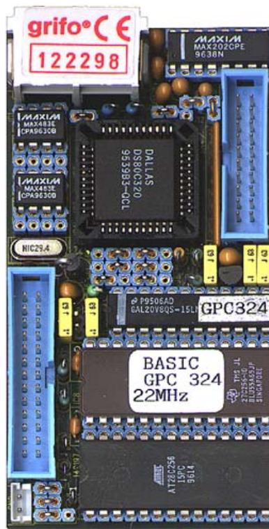
**FIGURE 8: SNAPSHOT OF A GPC® 324D**
