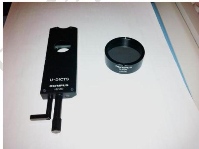
Figure 1-6: The lower DIC Prism and Upper Polariser
