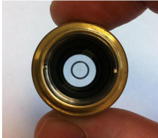
Figure 1-4: A phase plate inside an objective lens
