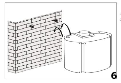
**6)** Hang the hood onto the support screws.
