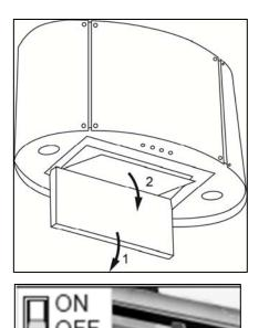
• Open the cover **(1)** that sits over the grease filter (as shown in the line drawing opposite).
