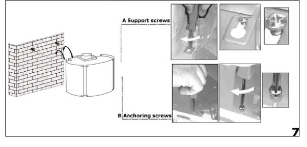
7) Fully tighten the support screws (A) and then screw the anchoring screws (B) through the relevant holes in the cooker hood. Fully tighten the anchoring screws into the wall.
