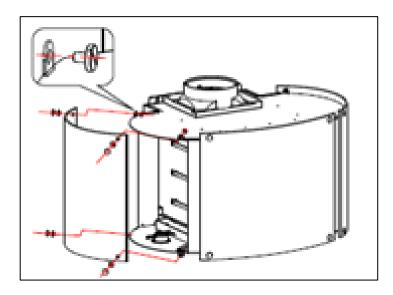
• The glass can be attached to the cooker hood using the four provided screws as shown in the picture above.
