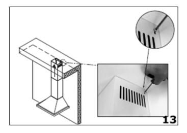
**13)** Lift chimney section **(D)** up to the ceiling and secure it to the L shaped bracket using the screws provided.
