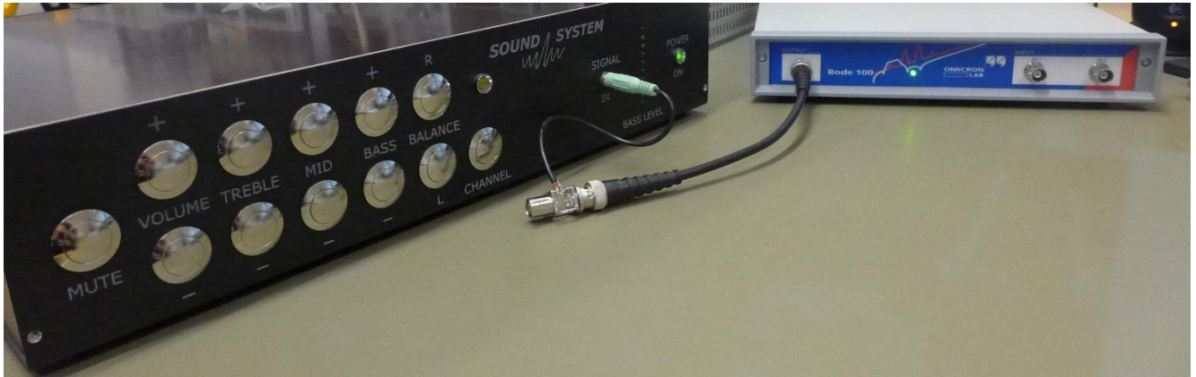
Figure 14: Standard input impedance measurement - connection setup
