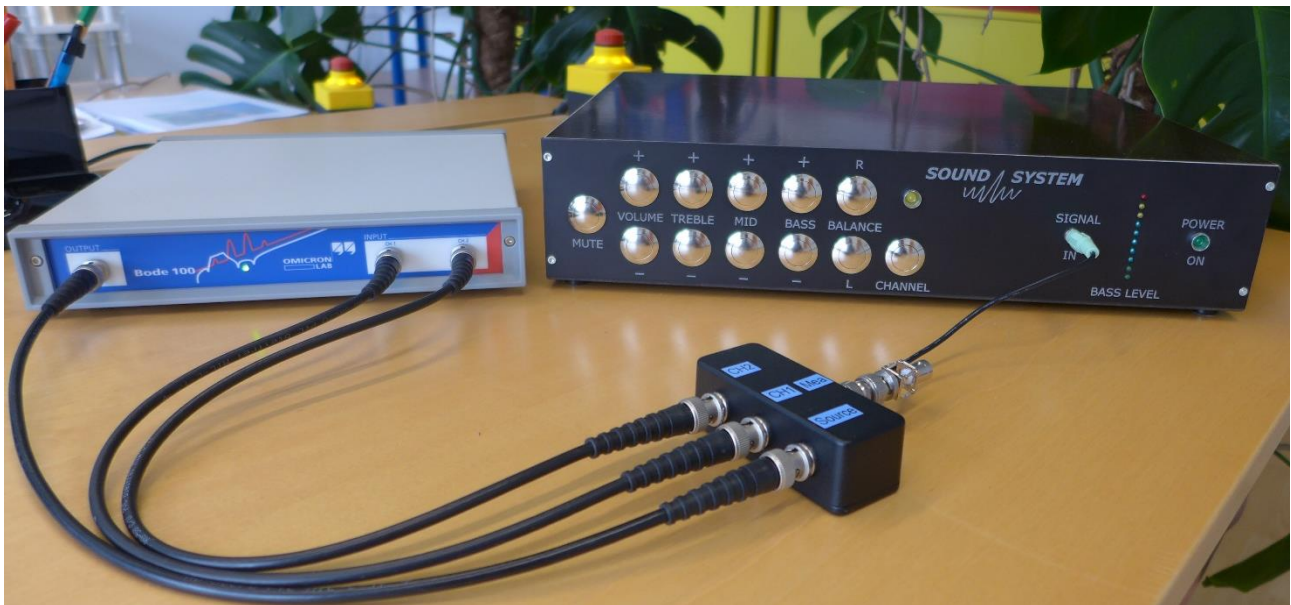
Figure 18: Input impedance with high impedance bridge - setup front view
