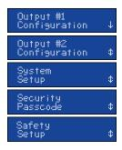
Press the Enter button to display the initial menu screen. This screen allows you to select which Output to configure, the System Setup, Security Passcode, and the Safety Setup. Each output has its own individual settings. All settings in the unit are stored in non-volatile eeprom memory which is retained during a power outage.
