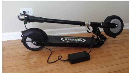
1. Turn the scooter off. The charge port (**K**) is located on the frame of the scooter above the folding mechanism. Open the charge port rubber protective cover and securely plug the charger into the charge port.
