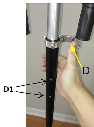
4. Open the handlebar's quick release lever (**D**). Raise the handlebar to the desired height until you hear it click and lock into place. (You have two handlebar heights to choose from (**D1**).) Lift up and push down on the handlebar to ensure it is securely locked into place. Close the quick release lever (**D**).
