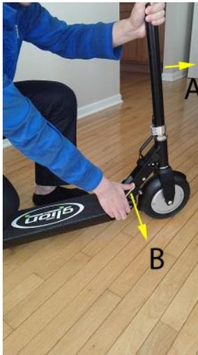
3. While pressing your knee on the board to secure the scooter, push the handlebar **(A)** slightly away from you (forward) to release the tension on the hook plate folding mechanism. Press down on the silver folding lever **(B)** and lower the handlebar down to the locked position. **Reminder: The folding lever will not move unless the handlebar is slightly pushed forward to release the tension on the hook plate folding mechanism.**
