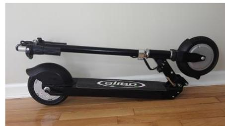
4. Closed view. Scooter is in locked position and ready to carry.
