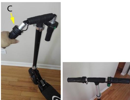
3. Lift the handlebar grips (**C**) until they lock into place. (You may do both at the same time.) Make sure both handlebars are securely retracted into the T bar.
