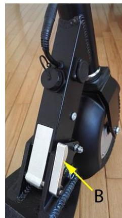
2. Push down on the silver lever (**B**) while simultaneously lifting the handlebar (**A**) up and forward. (Put one foot or knee on the board to steady the scooter as you push the neck forward.) Continue pushing forward until the mechanism locks into place.
