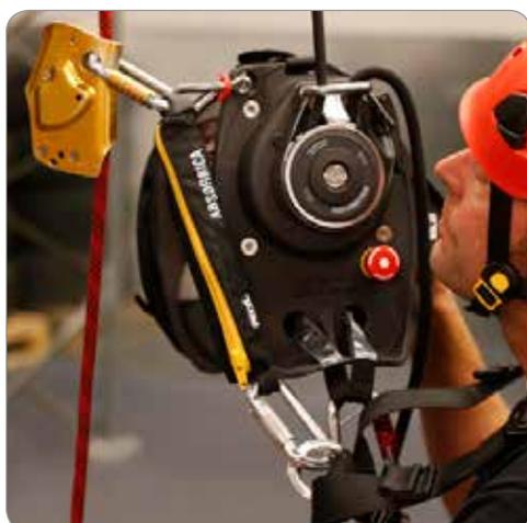
3) Connect the ascender to the low attachment point (EN 813) of the harness and connect the energy absorber of the backup to the fall arrest point (EN 361) and you are ready to go.
