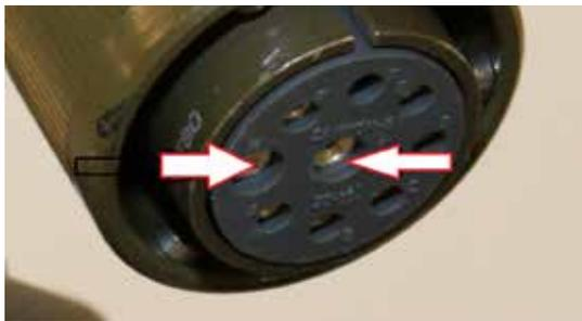
1) Measure the voltage (on pins I and H as shown in the picture) of the battery with a common voltmeter. It shall be 37,2 V when the battery is fully charged.
