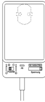
Fig. 5: Set wall-plug power supply to tip positive, 12 V. Switch arrangement and labeling may differ or be absent.
