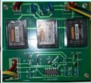
Z-Axis Controller Board
