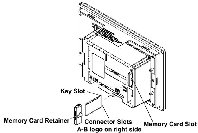
**Note:** The back of the PanelView 900 terminal is shown above. The location of the card slot will vary between the different terminals.
