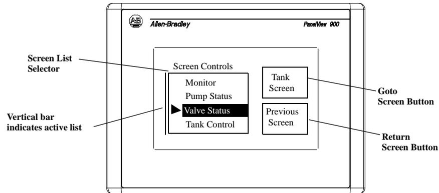
Goto and Return screen buttons can have a variety of appearances such as unique inner text, fill pattern, border or shape. Return screen buttons display the previous screen. Goto screen buttons display the assigned screen.
