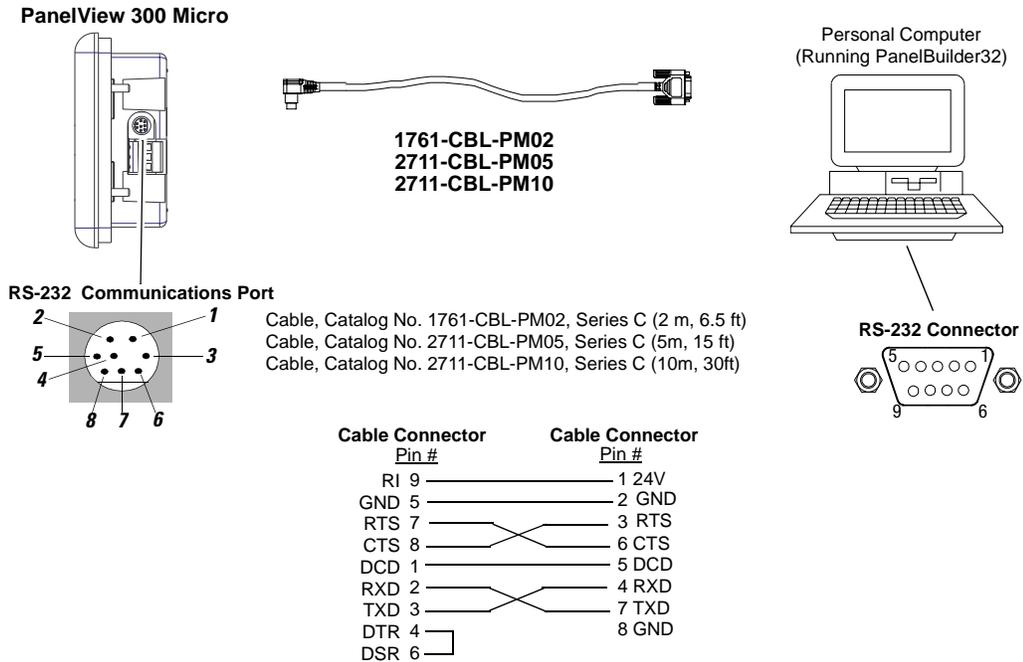
Refer to the PanelBuilder32 Software user manual for application download instructions. Here's a short summary of the methods that can be used to transfer files to a PanelView 300 Micro:
