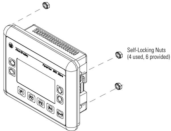
5. Alternately tighten the self-locking nuts until the terminal is held firmly against the panel. Tighten the nuts to a torque of 10 inch-pounds. Do not overtighten.
