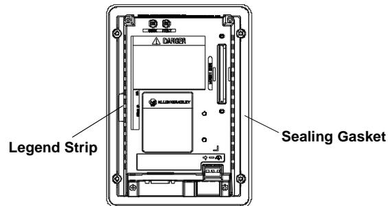
3. Verify that the end of the legend strip is fully inserted and does not interfere with the sealing gasket.
