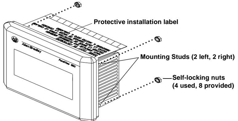
8. Alternately tighten the self-locking nuts until the terminal is held firmly against the panel. Tighten nuts to a torque of 10 inch-pounds. Do not over-tighten.
