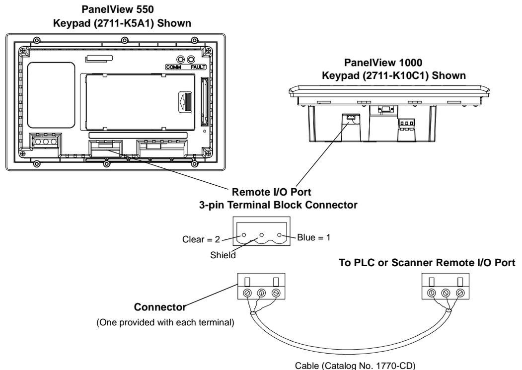
**Note:** The polarity of the Remote I/O Connector on the PanelView terminal is reversed from the PLC Scanner connector. However, the polarity is the same as the scanner card connection to the SLC.
