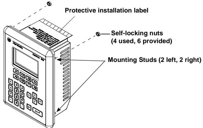
7. Alternately tighten the self-locking nuts until the terminal is held firmly against the panel. Tighten nuts to a torque of 10 inch-pounds. Do not over-tighten.
