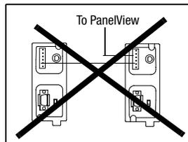
Do not connect the PanelView to Port 3 of the AIC+ when Port 3 is networked to other devices.
