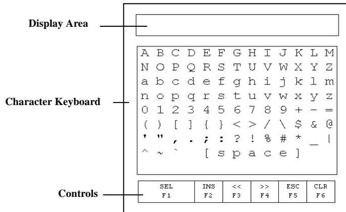
Select characters from the Character Keyboard by moving the cursor (with the keypad arrows) over a character and pressing the Sel-F1 function key. The character appears in the Display Area. This area scrolls so you can enter a string that is longer than the Display Area. All characters are sent to the controller even if not visible.
