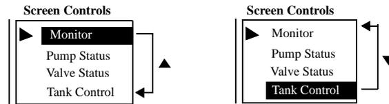
If a screen list contains more items than can appear at one time, the list scrolls. If the cursor is at the top or bottom of a scrolling list, the list scrolls one row at a time as the Up/Down arrows are pressed.
