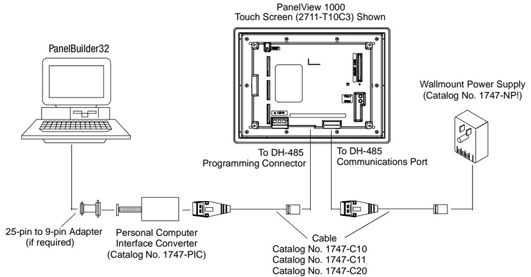
**Connecting a Computer to DH-485 Connector using a DH-485 Powered Device**
