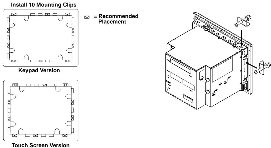
6. Alternately tighten the mounting clip screws until the terminal is held firmly against the panel. Tighten mounting screws to a torque of 10 inch-pounds. Do not over-tighten.
