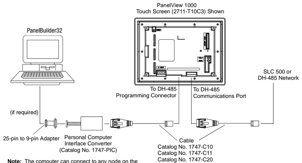
**Note:** The computer can connect to any node on the network. It is not necessary to directly connect the computer to the PanelView terminal.
