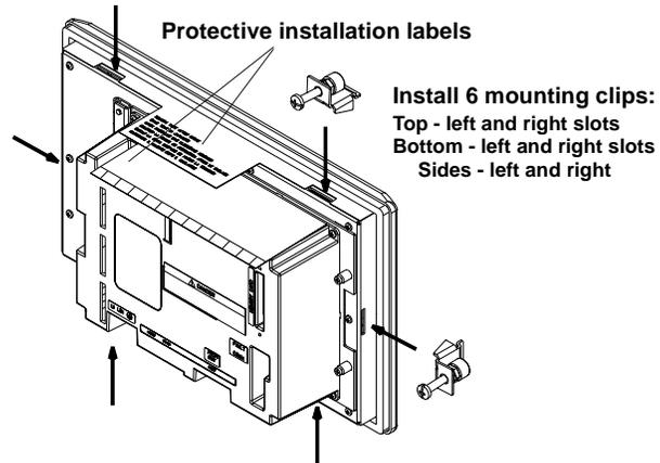
6. Alternately tighten the mounting clip screws to a torque of 10 inch-pounds. Do not over-tighten.
