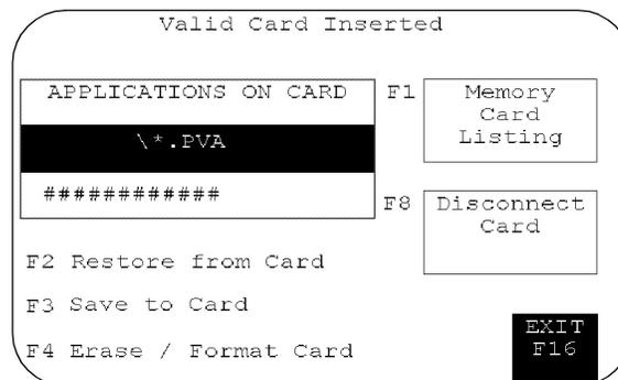
4. Press Memory Card Listing, [F1] on keypad terminals, until the application file you want to load is displayed.
