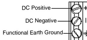
Use #16 to #22 AWG Solid Wire or #18 to #22 AWG Stranded
