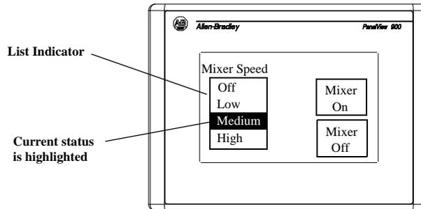
An indicator list may have a maximum of 255 entries. The list automatically scrolls to display the status of an item. **Note:** List indicators do not have a cursor ► like control or screen selector lists.
