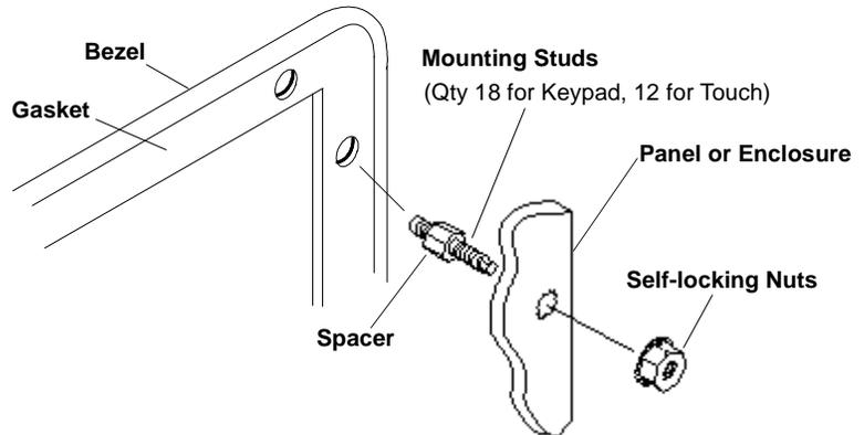
3. Make sure the sealing gasket is properly positioned on the terminal. This gasket forms a compression type seal (NEMA Type 4). Do not use sealing compounds
