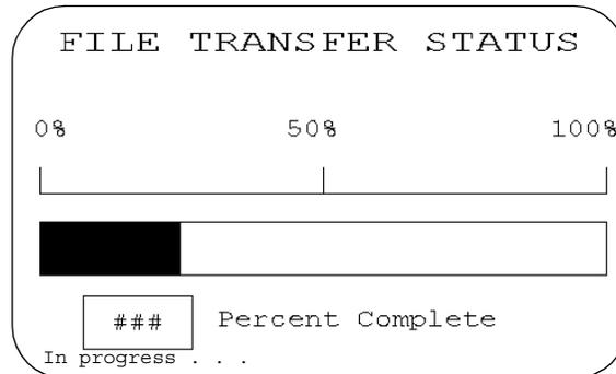
6. When the transfer is complete, the PanelView terminal checks the validity of the application, resets and runs the application.
