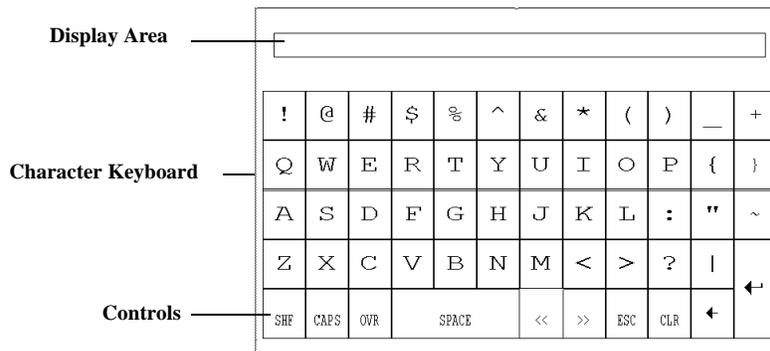
Select characters by touching the Character Keyboard on the screen. The character is entered in the Display Area. This area scrolls so you can enter a string that is longer than the Display Area. All characters are sent to the controller even if not visible.
