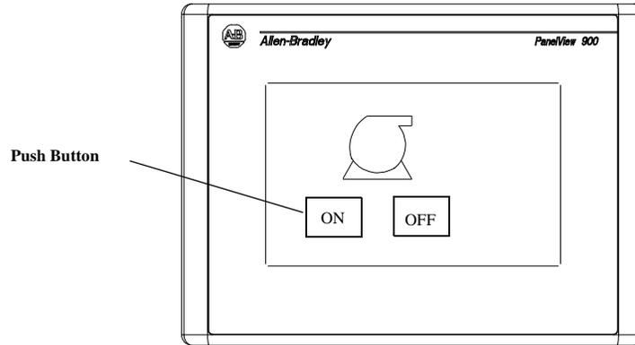
Push buttons have a variety of appearances. Push buttons may change their inner text, fill pattern, border or shape when pressed (each state assigned different attributes).
