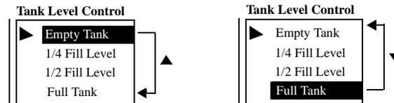
If the list contains more items than can appear at one time, the list scrolls. If the cursor is at the top or bottom of a scrolling list, the list scrolls one row at a time as the arrow keys are pressed.
