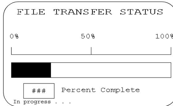
6. When the transfer is complete, the application file name appears in the Applications on Card list. Press Memory Card Listing, [F1] key on keypad terminals, to scroll through the list.
