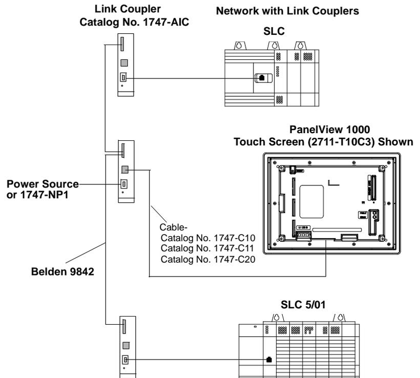
**Important:** The DH-485 network cable requires proper shielding, grounding and termination. Refer to Data Highway / Data Highway Plus / Data Highway-485 Cable Installation Manual (Publication No. 1770-6.2.2).
