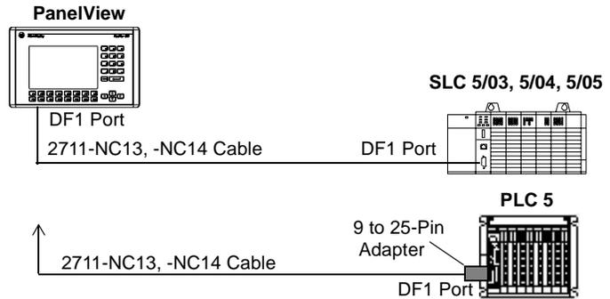
Use an optical isolator or equivalent when grounding level differences exist between the controller or modem and the PanelView.
