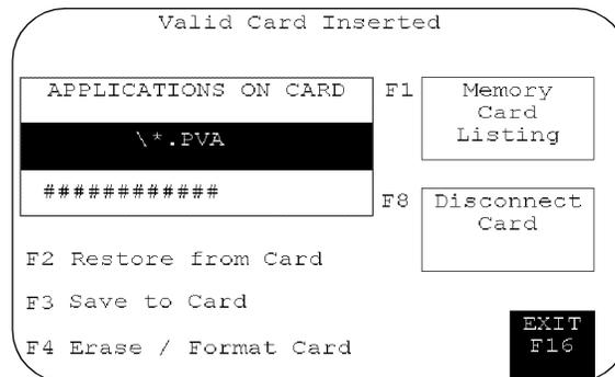
4. If necessary, press Erase/Format Card, [F4] key on keypad terminals, to format or erase a 2711-NM11, -12, -13, -14 memory card. Do not perform this operation on a 2711-NM2xx ATA card (where xx is size in megabytes). The card becomes inoperable. Because this operation erases all data on the memory card, you are prompted to abort or continue.
