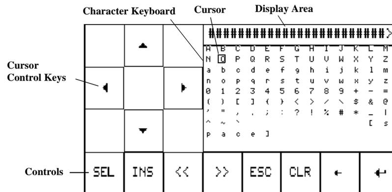
To select characters from the Character Keyboard, press the cursor control keys to move the cursor over a character and then press the SEL key. The character is entered in the Display Area. This area scrolls so you can enter a string that is longer than the Display Area. All characters are sent to the controller even if not visible.
