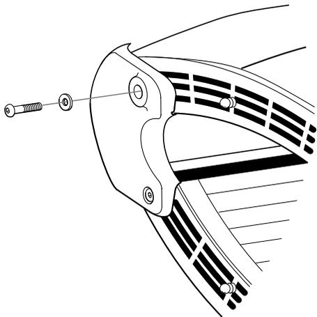
2. Insert the 5/16" x 1 1/2" bolts with the nylon washers into both hinge brackets. Tighten bolts into the end-cap threaded inserts until snug, then an additional half turn. Do not over-tighten to avoid damaging threaded inserts.
