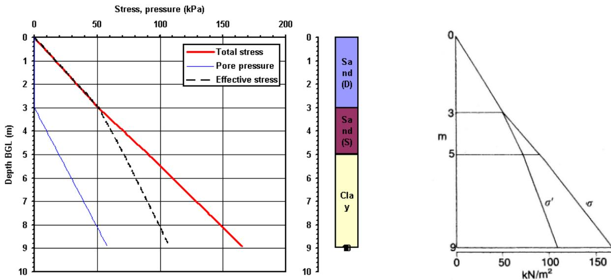
Figure 4: Comparison stress profiles from (a) Stress\_CSM8 and (b) main text, Figure 3.2
